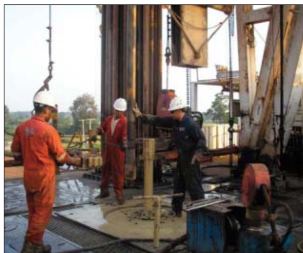
Triples (photo on left) are stacked on the drill floor of Rig GW-80 in Thailand (Fig. 2). Drill crew (photo on right) runs pipe on Rig GW-80 (Fig. 3). Photos provided by GWDC Thailand.
