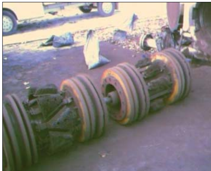
Dual module bidirectional pigs with brushes continued to remove large amounts of black powder even after other techniques had been applied. The interior of the pipeline on the Bulgarian side of the border was not protected with coating (Fig. 4).
